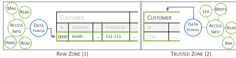
Figure 3. The image displays access metadata collected on varying granular levels of the customer table. The customer table is stored twice, once in each data lake zone. The green circles are metadata objects with properties, e.g., a user object with the name “Max”. They belong to the accordingly highlighted part of the table. The blue circles denote a pointer containing the data’s storage location. (Colored figure online)
